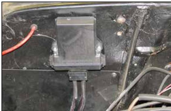
4. Connect the wiring harness to the control unit.
