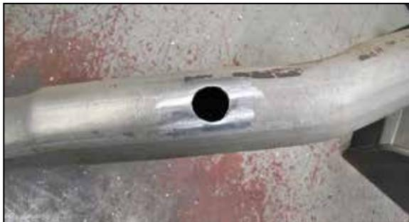
3. Drill a 3/4" id hole in the marked location. Deburr the hole after drilling.
