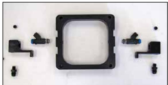
4. Assemble the ECI injector plate. The injector(s) and fuel rail(S) can be installed two different ways onto the injector plate. It is advisable to mock up your installation on the engine to determine the best position for your injector(s) and fuel line(s) to be routed. Once you have determined the best position for your situation, install the injector(s), Fuel rail(s), fuel line fitting(s) and plug(s) into the injector plate.
