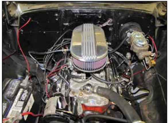
9. Reinstall the air filter assembly.
