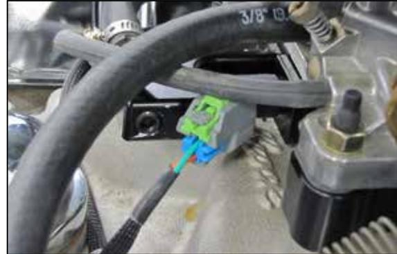
5. Route the wiring pigtails for the injector(s) and other optional connections so they will not interfere with mechanical assembly or exhaust and then connect them to the injector(s) and optional locations.
