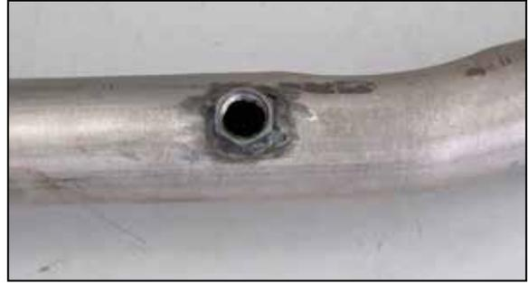
4. Weld the provided O2 sensor fitting into the exhaust pipe.
