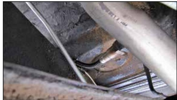
5. Install the provided O2 sensor into the fitting.
