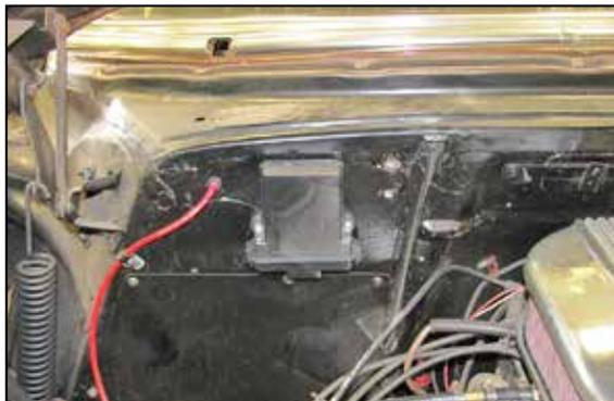
3. Drill the holes and mount the control unit in the desired location.
