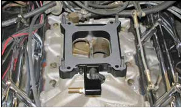
5. Install the assembled injector plate and new carburetor base gaskets onto the intake manifold.
