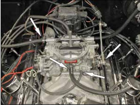
1. Turn off the ignition and disconnect the negative battery cable and remove the air filter assembly. Label all the vacuum lines prior to disconnecting for ease of reassembly, i.e. vacuum advance, brake booster. Disconnect the throttle linkage, fuel line, vacuum lines, electrical wiring etc. from the carburetor. Be sure to capture any fuel that may leak out of the fuel line. Pay close attention to any lines that may be damaged, replace them at this time.
