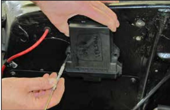
2. Find a suitable location to mount the EC1 control unit that is away from direct heat, wet conditions and any mechanical interference. Place the control unit in position and mark the location for holes to be drilled.
