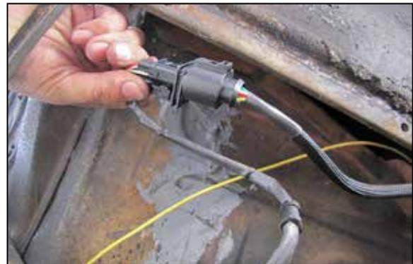
6. Connect the O2 sensor pigtail into the ECI wiring harness.
