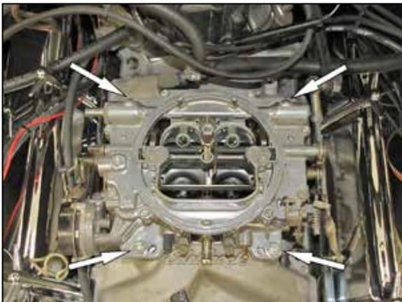
2. Remove the bolts that secure the carburetor to the intake manifold. Remove the carburetor and gasket from the manifold.
