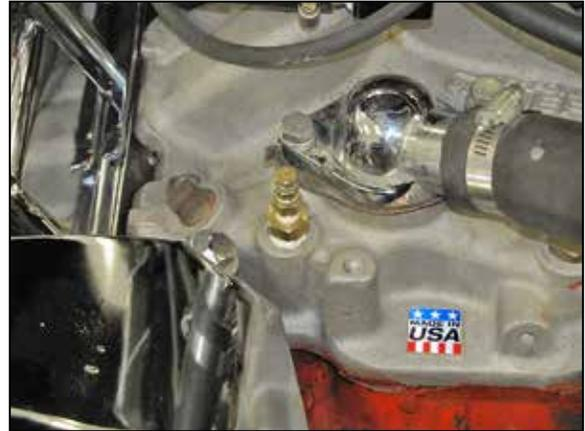
8. If you desire to connect a coolant temperature sensor to the system, find a suitable location in the cooling system to install the coolant temperature sensor. Usually this will be in the intake manifold near the thermostat housing.
