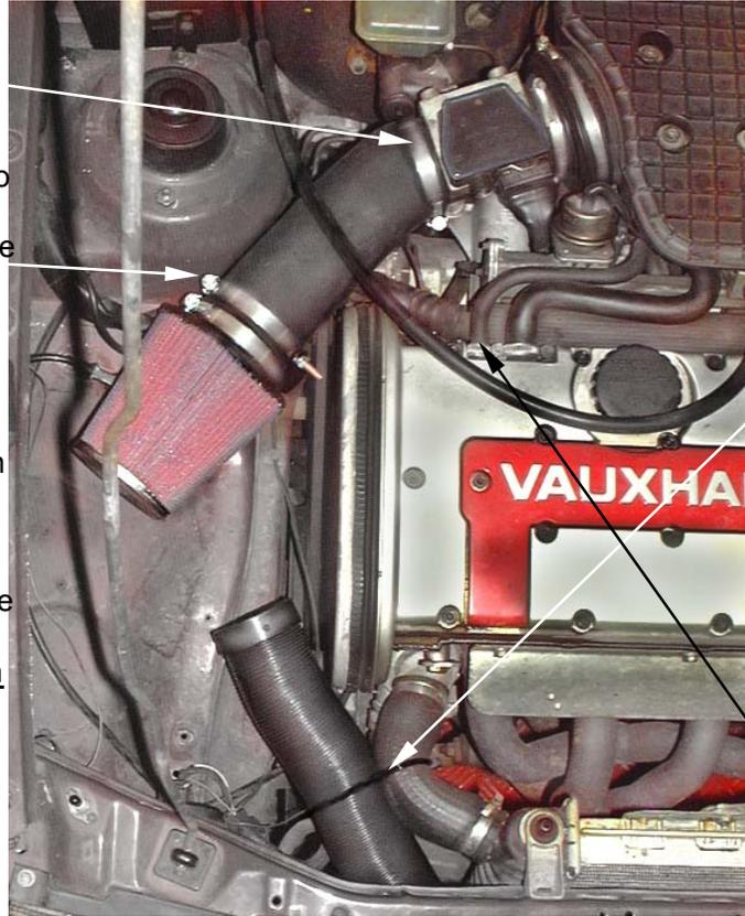
5. Carefully lengthen the flexi cold air hose to approx. 46cm / 18", pierce a 3mm hole in one end of the hose and feed a long plastic tie through the hole. Feed the end of the hose past the radiator to the front grille. Attach the other end of the cold air hose to the top coolant hose using a long plastic tie supplied. Position the end of the flexi cold air hose to finish **10cm / 4"** from the filter **no nearer.** **Note: Ensure that the flexi hose clears all belts and pulleys.**
