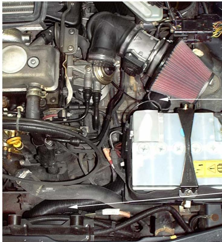
3. Attach the flexi cold air hose to the original mounting bracket with a long plastic tie. Point the top of the cold air hose at the filter so it is no nearer than **10cm / 4"** from the filter.
