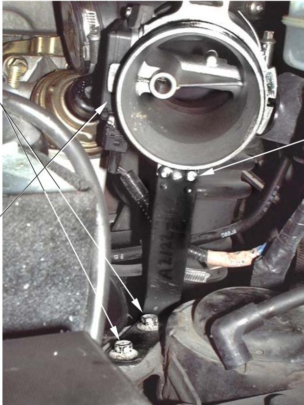
3. Attach the MAS to the new mounting bracket.
