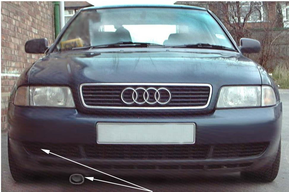
Pierce / drill a 3mm hole in the end of the cold air hose and feed the hose down to the front lower side vent in the front bumper (It may be necessary to reposition the horn mounting bracket). Pierce / drill a 3mm hole in the plastic vent trim, ovalise the end of the hose and secure the hose to the trim using a long plastic tie. (Alternatively, feed the hose down to the lower spoiler trim and secure the hose to the trim using a long plastic tie).
