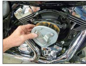
5. Remove the air filter from the vehicle and disconnect the crankcase breather tubes.
