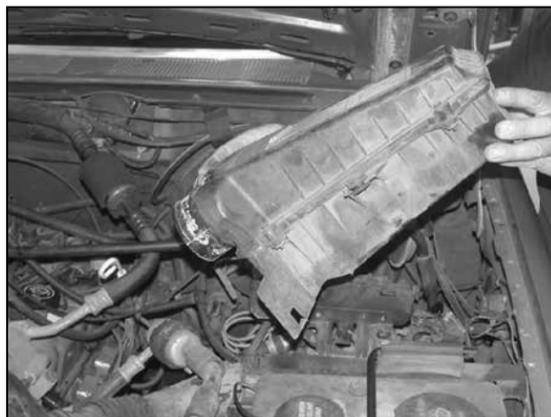
5. Remove the crank case vent from air box then remove the two 8mm bolts that retain the air box to vehicle. Then remove air box from vehicle as shown.
