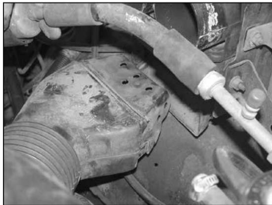
4. Remove the fresh air intake tube from the bottom of air box as shown.
