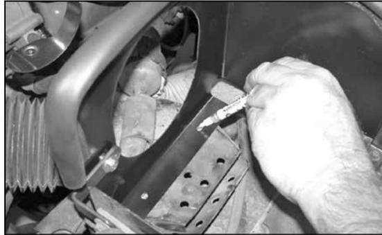
12. Install the heat shield onto the vehicle then line up the fresh air duct to the heat shield and mark the two holes with a marker, then remove heat shield from vehicle.
