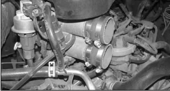
8. Secure the provided silicone hoses (08405) onto the throttle body with the provided hose clamps as shown.
