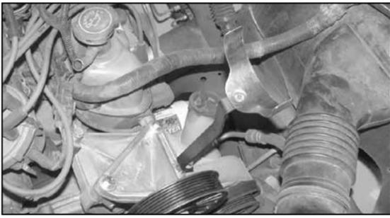
7a. On vehicles that do not come equipped with A/C, mount the saddle bracket assembly from step 6a onto the idler pulley bracket as shown.
