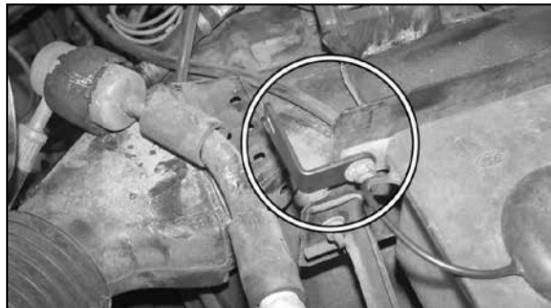
11. Remove the nut that retains the coolant tank to vehicle then mount the provided bracket (070932) to tank with the nut that was removed.
