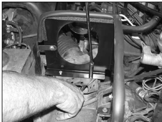
14. Re-install the heat shield onto the vehicle then mount the fresh air duct to the heat shield with the provided hardware as shown.
