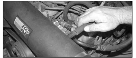
16. Remove the crank case vent tube from valve cover then connect the provided silicone hose to the valve cover, then connect to the intake tube as shown. Trim hose for best fit.
