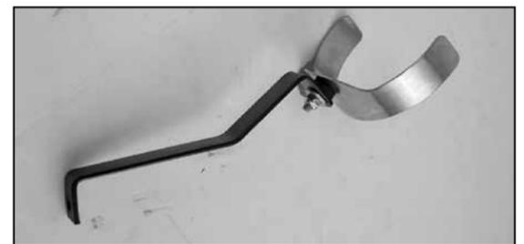
6a. On vehicles that do not come equipped with A/C, assemble the saddle bracket onto bracket (07165) as shown.
