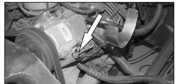
7. On vehicles that come equipped with A/C, remove the front lower A/C mounting bolt. Then secure the saddle bracket assembly from step 6 onto vehicle as shown.
