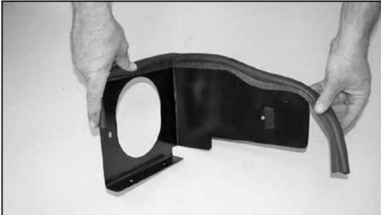
9. Install edge trim onto heat shield as shown. Trim if needed.
