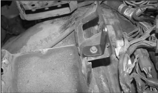
10. Install the provided bracket (07879) onto the air box mounting bracket as shown using one of the bolts that was removed in step 5.
