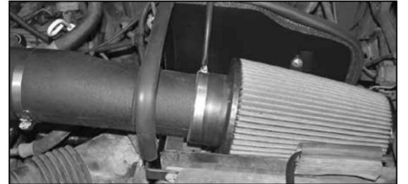
17. Install the air filter onto the new intake tube as shown.
