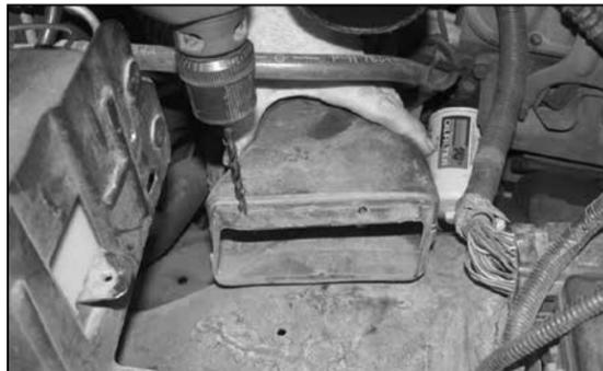
13. Remove the heat shield and drill two 1/4" holes were you marked in the previous step.
