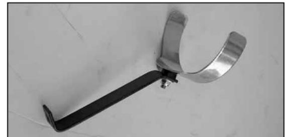
6. On vehicles that come equipped with A/C, assemble the saddle bracket onto bracket (07164) as shown.
