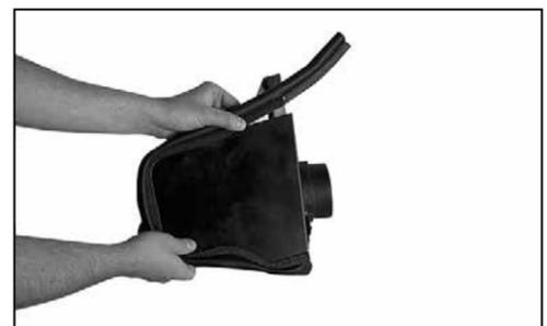
8. Apply the trim seal to the heat shield assembly as shown.
