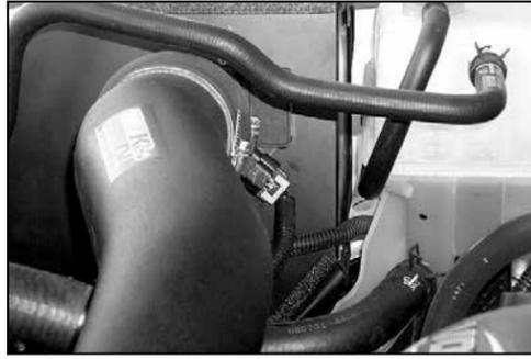
16. Reconnect the mass air sensor electrical connection as shown.
