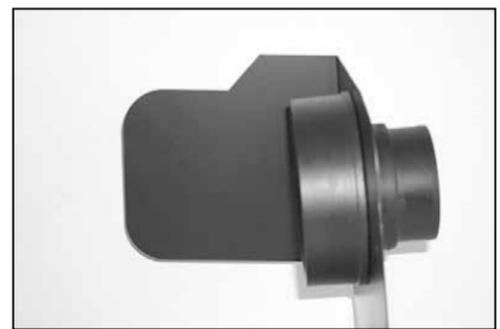
7. Assemble the mass air adapter, heat shield, gaskets and the mass air sensor as shown above.
