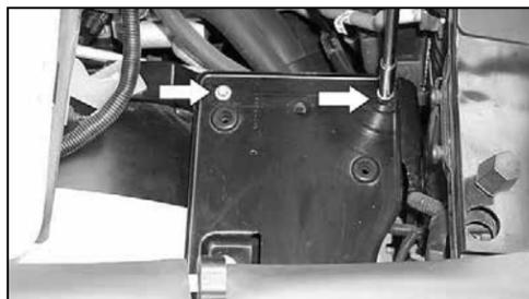
5. Loosen and remove the two air cleaner mounting tray bolts as shown.
