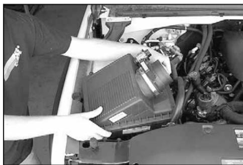
4. Pull firmly upwards to release the air cleaner assembly from the mounting tray grommets, then remove the assembly.
