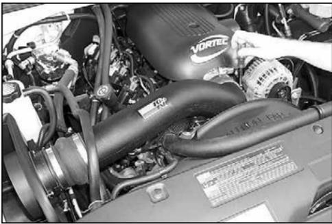
12. Install the K&N® intake tube onto the mass air sensor, then secure the other end onto the throttle body as shown.
