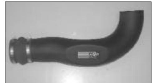
11. Install the silicone hump hose (08176) and hose clamps onto the K&N intake tube as shown.
