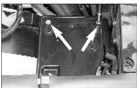
5. Loosen and remove the two air cleaner mounting tray bolts as shown.
