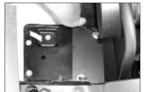
13. Adjust the heat shield and intake tube for best fit, then tighten the two hex bolts as shown.
