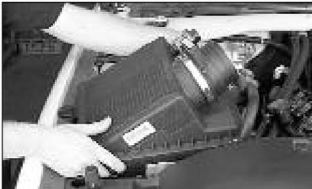
4) Pull firmly upwards to release the air cleaner assembly from the mounting tray grommets, then remove the assembly.
