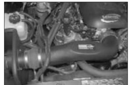
12. Install the K&N intake tube onto the mass air sensor, then secure the other end onto the throttle body as shown.
