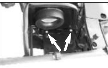
9. Install and mount the heat shield assembly to the air cleaner mounting tray using the bolts removed in step 5.
