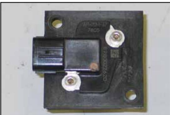
10. Install the mass air sensor into the adapter and secure with the provided hardware.
