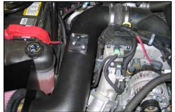
21. Install the K&N® Intake Tube into the silicone hose at the turbo inlet and into the heat shield, then secure the K&N® Intake Tube with the provided hose clamp and hardware as shown.
