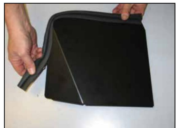
23. Install the 20" piece of edge trim onto the filter cover as shown.
