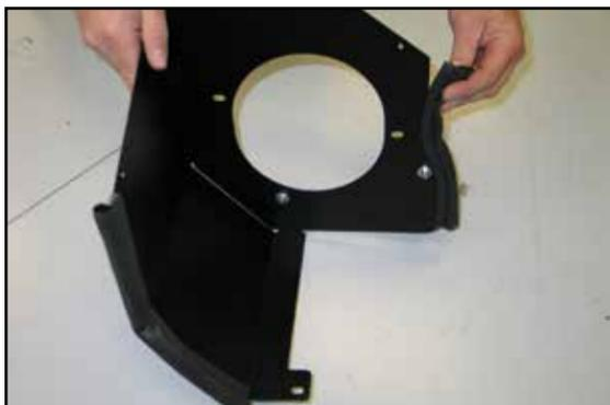
18. Install the remaining 11" edge trim onto the heat shield as shown.
