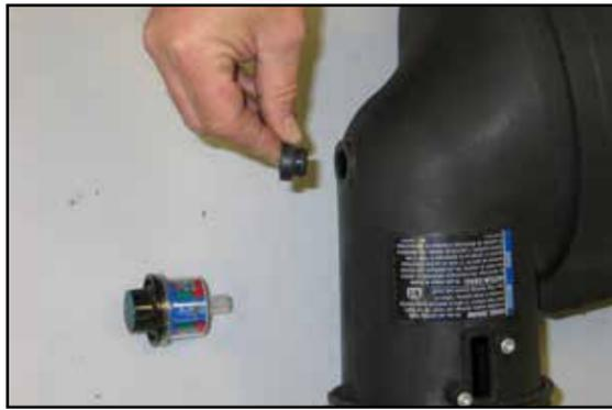
13. Remove the filter minder and grommet from the stock intake tube as shown.
