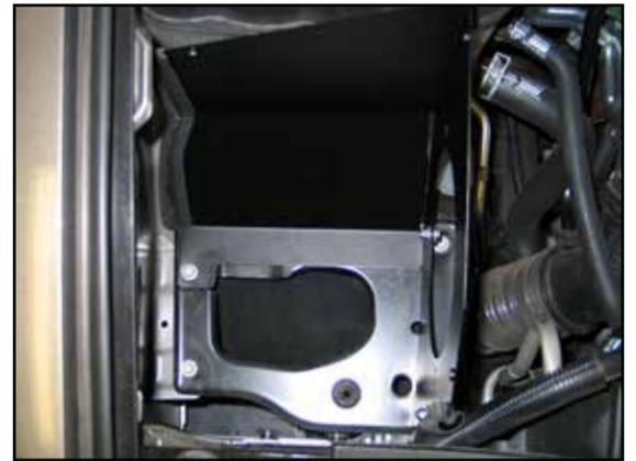
19. Install the Heat shield assembly onto the factory air box mounting plate and secure with the factory bolts removed in step #7.
