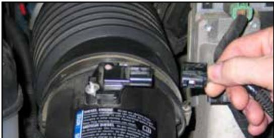
2. Depress the locking tab and then disconnect the Mass air sensor electrical connection.
