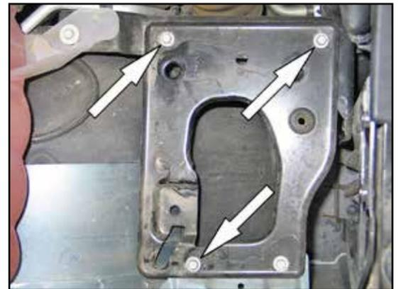
7. Remove the three air box mounting plate bolts shown.
