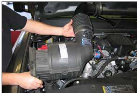
4. Disconnect the stock intake tube from the turbo inlet tube and then lift the complete stock intake assembly from the vehicle as shown.
