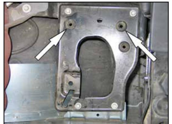
6. Remove the two air box mounting grommets shown from the air box mounting plate.
