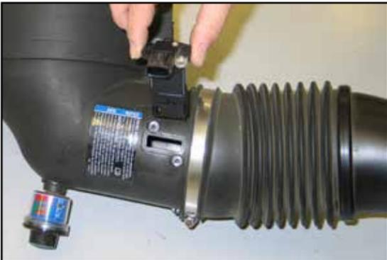
9. Remove the two screws that secure the mass air sensor onto the stock intake tube and then remove the mass air sensor as shown.
