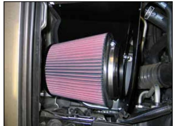
20. Set the K&N® Air Filter into the heat shield as shown.
