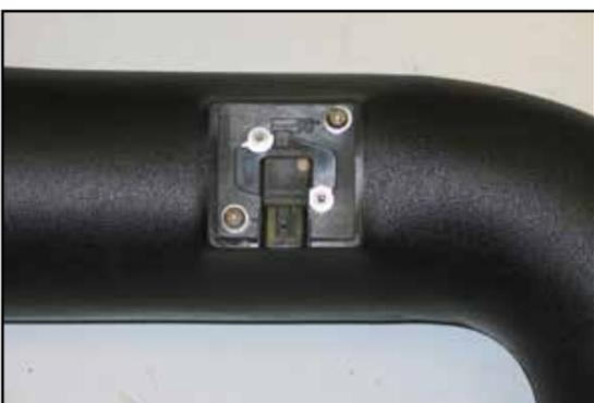
12. Secure the mass air sensor assembly to the K&N® Intake Tube with the provided hardware.
