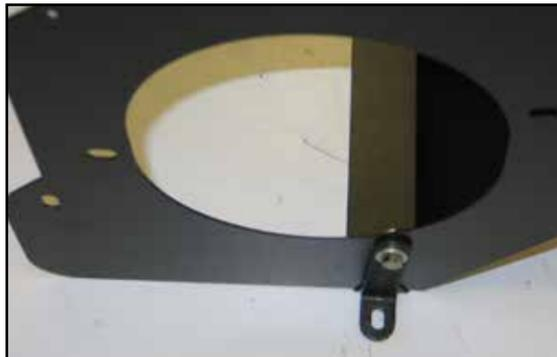
15. Install the "L" bracket (07805) onto the heat shield as shown with the provided hardware.
