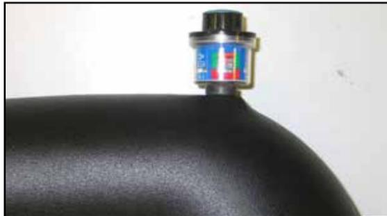
14. Install the filter minder and grommet into the K&N® Intake Tube as shown.
