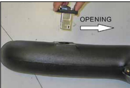
11. Install the mass air sensor assembly into the K&N® Intake Tube.
