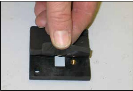
8. Install the provided gasket onto the mass air sensor adapter as shown.
