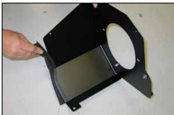
17. Install one of the 11" edge trims onto the heat shield as shown.
