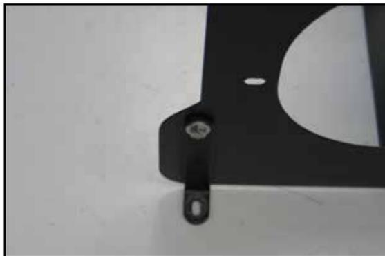
16. Install the "L" bracket (070952) onto the heat shield as shown using the provided hardware.
