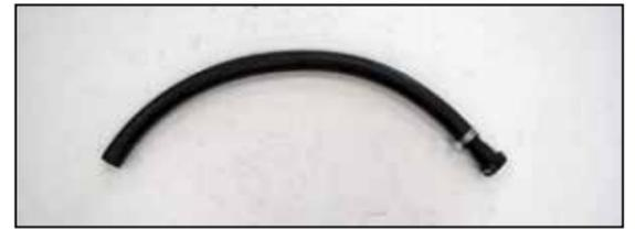
15a. For HELLCAT REDEYE models, assemble the quick connect fitting and crank case vent hose provided as shown.
