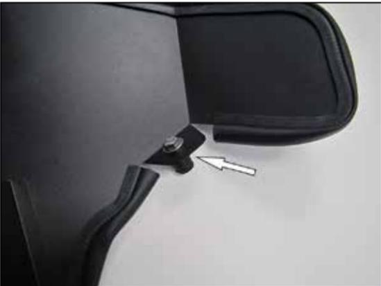
8. Install the nut insert onto the heat shield and secure with the provided hardware.
