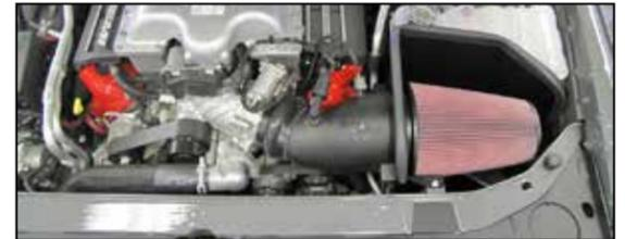
16. Install the K&N® air filter onto the filter adapter and secure with the provided hose clamp.
