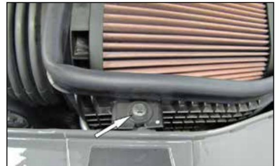
4. Remove the bolt that secures the air filter housing to the core support.
