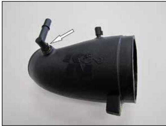
11. Install the provided 90° quick disconnect fitting into the K&N® intake tube as shown.
