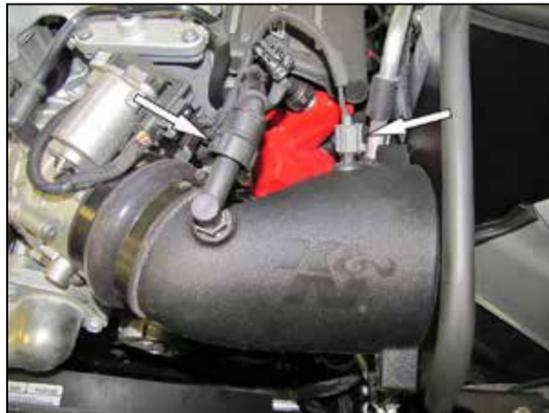
15. Reconnect the inlet air temperature sensor electrical connection. On 2018 DEMON models connect the crank case vent quick connect fitting to the fitting installed into the K&N® intake tube.
