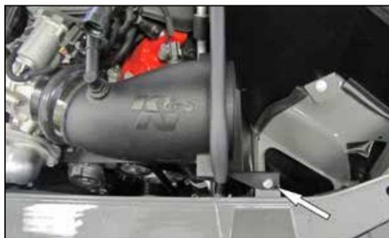
14. Secure the heat shield to the core support with the provided hardware then secure the intake tube with the provided hose clamp.
