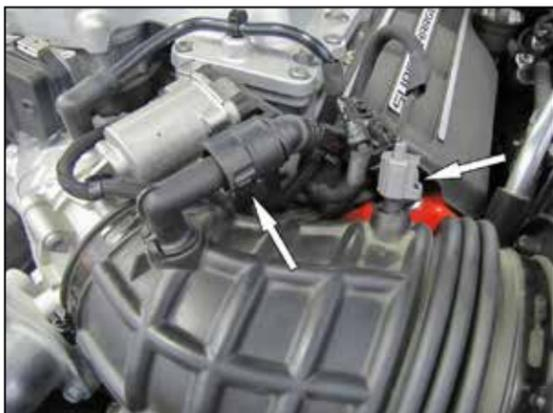
2. On 2018 DEMON models, disconnect the crank case vent line quick disconnect fitting and inlet air temperature sensor electrical connection. On HELLCAT REDEYE models disconnect the inlet air temperature sensor electrical connection only.
