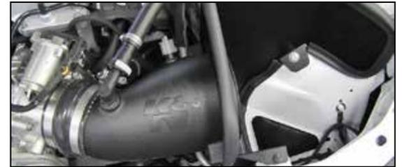
15b. Install the assembled crank case vent assembly onto the quick connect fitting installed into the K&N® intake tube and then connect the other end to the factory shut off valve and secure with the provided hose clamps.
