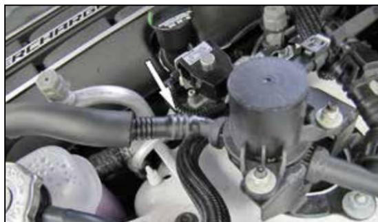
2a. On HELLCAT REDEYE models, use a razor knife or similar tool to slice the crank case hard line to enable it to be disconnected from the shut-off valve.
