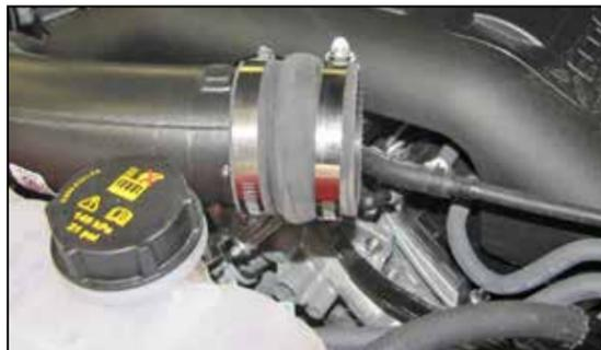
15. Install the provided coupling hose (087121) onto the passenger side turbo inlet tube and secure with the provided hose clamp.
