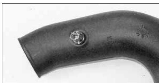
18. Remove the O-Ring from the inlet air temperature sensor, then install it into the grommet installed into the K&N® intake tube.
