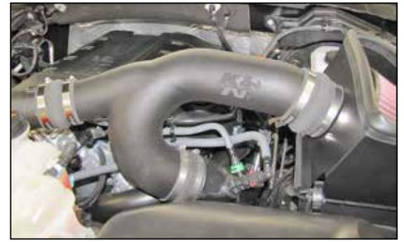
19. Install the K&N® intake tube into the turbo inlet hoses and then into the hose at the throttle body, adjust the tube for best fit and then secure with the provided hose clamps.
