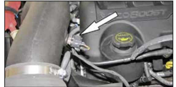
20. Reconnect the inlet air temperature sensor electrical connection.
