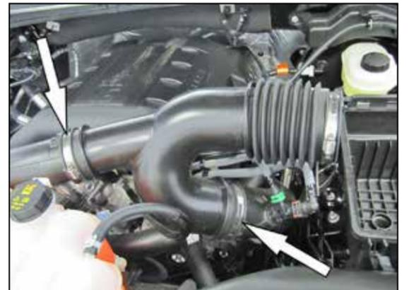
6. Loosen the hose clamps securing the intake tube to the two turbo inlet tubes and then remove the intake tube from the vehicle.
