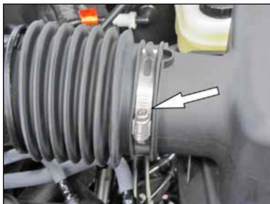
3. Loosen the hose clamp securing the factory intake tube to the air filter housing.
