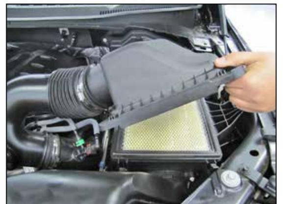
5. Lift up and remove the upper air filter housing and factory air filter.
