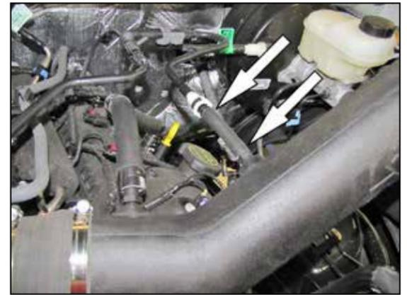
17. Install the quick disconnect union into the mating EVAP quick disconnect fitting and then connect the open EVAP vent hose to the fitting installed into the K&N® intake tube.
