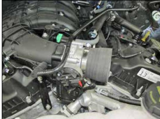
13. Install the provided step coupler hose (084055) onto the throttle body and secure with the provided hose clamp.
