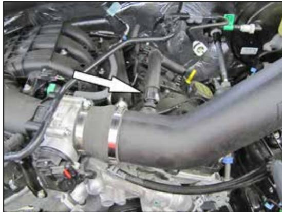
15. Connect the crank case vent quick disconnect fitting to the mating quick disconnect fitting installed into the K&N® intake tube.
