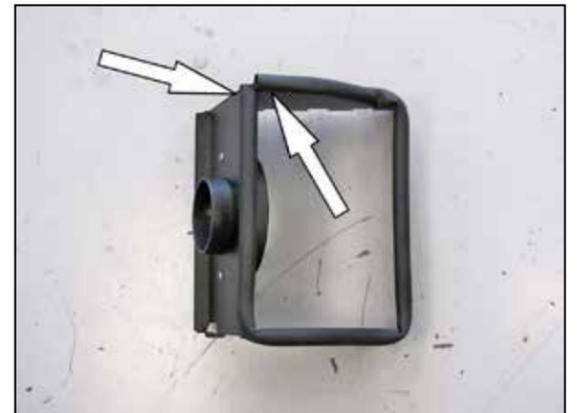
6. Install the provided bulb edge trim onto the heat shield as shown.
