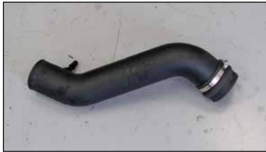
12. Install the provided hump coupler hose (08699) onto the K&N® intake tube and secure with the provided hose clamp.
