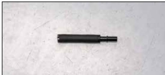
16. Install the provided EVAP vent hose onto the provided quick disconnect union as shown.
