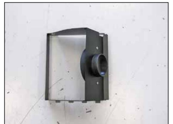
5. Install the filter adapter into the K&N® heat shield as shown and secure with the provided hardware.
