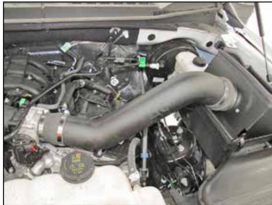
14. Install the K&N® intake tube assembly into the hose at the throttle body and onto the filter adapter, align the tube for best fit and then secure with the provided hose clamp.
