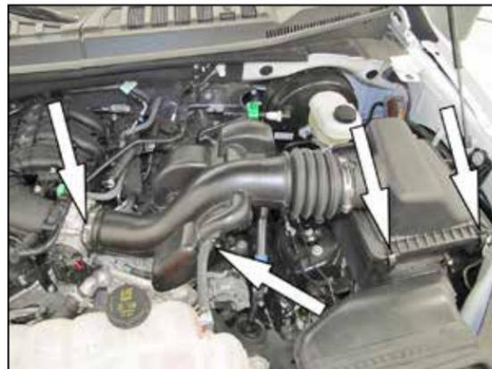
4. Loosen the hose clamp securing the intake tube to the throttle body, unhook the coolant reservoir hose from the intake tube and unclip the two upper air filter housing retaining clips. Then remove the upper air filter housing and intake tube assembly.
