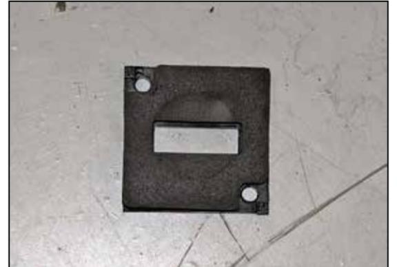
19. Install the gasket on to the K&N® mass air sensor adapter.
