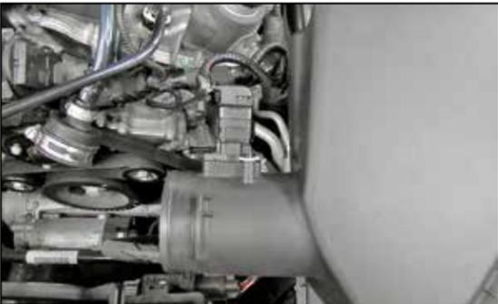
9. Disconnect the mass air sensor electrical connection.
