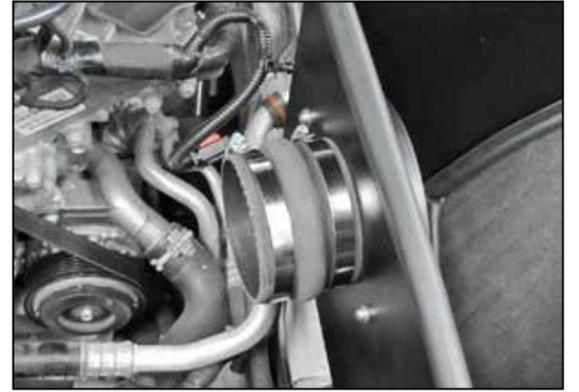
18. Install the provided hump coupler (08699) onto the filter adapter and secure with the provided hose clamp.
