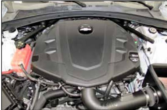
31. Reinstall the decorative engine cover and secure with the factory bolt and oil cap.
