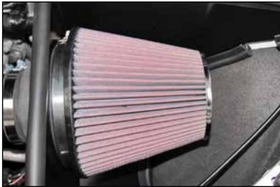
30. Install the K&N® air filter and secure with the provided hose clamp.
