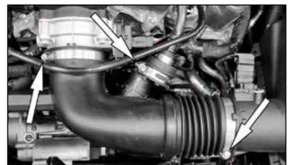
5. Loosen the three hose clamps that secure the intake tube and crank case vent tube then remove the intake tube from vehicle.
