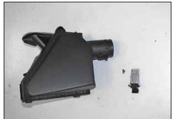
20. Remove the mass air sensor from the factory air filter housing.
