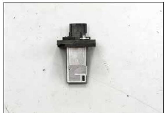
21. Install the mass air sensor into the K&N® mass air sensor adapter and secure with the provided hardware.
