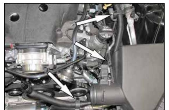
6. Release the three flexible clamps that secure the sound tube and disconnect the sound drum from the rear sound tube then remove the sound tube assembly.
