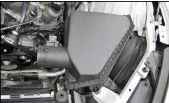
10. Lift up and remove the factory air filter housing assembly.
