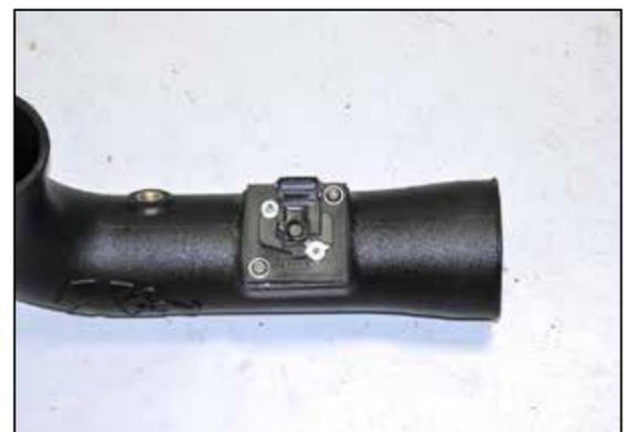
22. Install the mass air assembly into the K&N® intake tube as shown.
