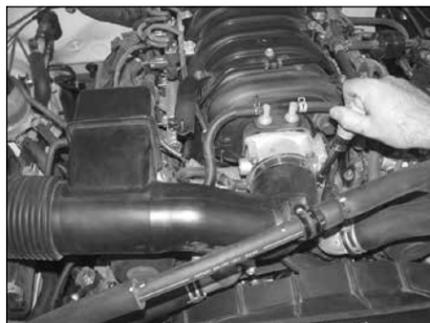
5. Loosen the hose clamp, which secures the stock intake tube to the throttle body
