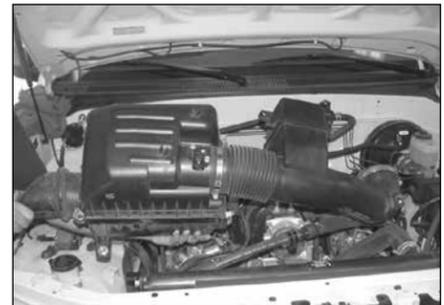
8. Remove the complete intake assembly from the vehicle as shown.
