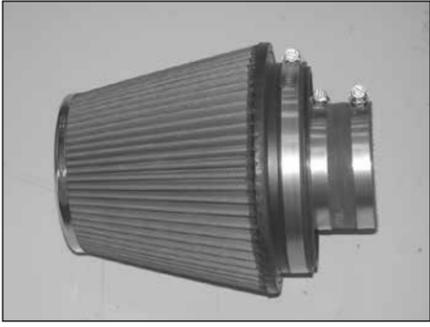
27. Install the silicone hose (08630) onto the filter adapter as shown and secure with the provided hose clamp.
