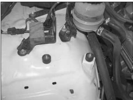
14. Install the two rubber mounted stud to the original airbox mounting holes as shown.
