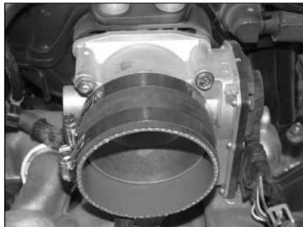
18. Install the silicone hose (08630) onto the throttle body and secure with the provided hose clamp as shown.
