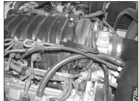
24. Install the provided fuel pressure regulator vent hose onto the fuel pressure regulator and then attach to the intake tube as shown.
