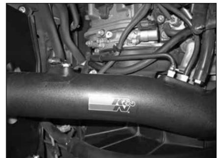
25. Attach the power steering pressure switch vent hose to the intake tube as shown.
