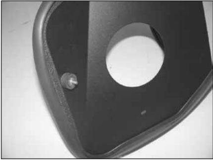
12. Install the rubber mounted studs onto the heat shield as shown using the provided hardware.
