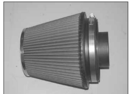
26. Install the filter adapter into the air filter as shown and secure with the provided hose clamp.
