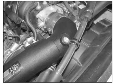
21. Attach the A/C hose to the intake tube with the bolt removed in step #4.
