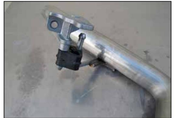
7. Install the driver side muffler hanger onto the K&N® tail pipe hanger.
