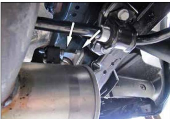
3. Loosen and remove the two bolts that secure the driver side muffler hanger to the chassis. **NOTE: one bolt is not in view in this picture.**
