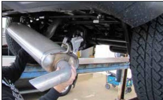
5. Using a twisting motion so the muffler pipe slides off the exhaust pipe, remove the muffler assembly from the vehicle. **NOTE: K&N Engineering, Inc., recommends that customers do not discard factory exhaust.**
