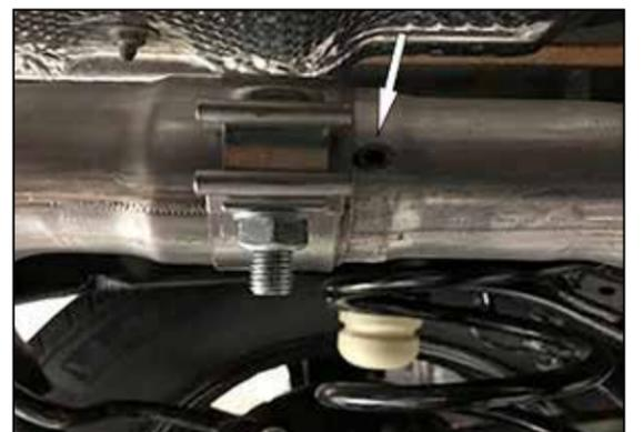
9. Make sure the K&N® tailpipe rests up against the clocking feature on the factory mid-pipe.
