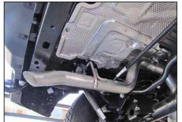
8. Install the K&N® tail pipe onto the factory exhaust pipe.
