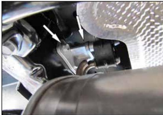
4. Loosen and remove the two bolts that secure the passenger side muffler hanger to the chassis. **NOTE: one bolt is not in view in this picture. Support the muffler assembly while removing the bolts as it may now swing and fall.**
