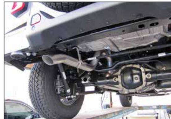
11. Check alignment and reposition as necessary. Once final position is satisfactory, tighten all band clamps from front to rear of vehicle.
