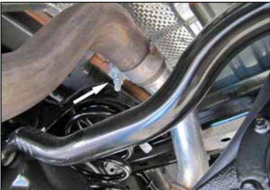
2. Loosen the clamp that secures the muffler pipe to the exhaust pipe.
