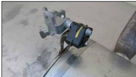
6. Remove the driver side muffler hanger from the stock muffler. **NOTE: if necessary, apply a small amount of lube to aid in the removal of the hanger.**
