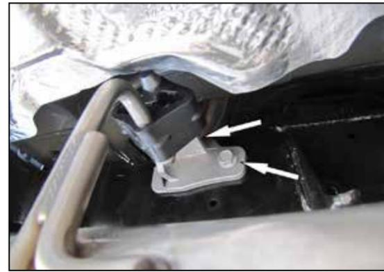
10. Secure the hanger to the factory location using the factory bolts removed in step #3.
