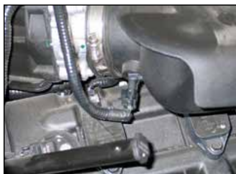
3. Disconnect the inlet air temperature sensor electrical connection.
