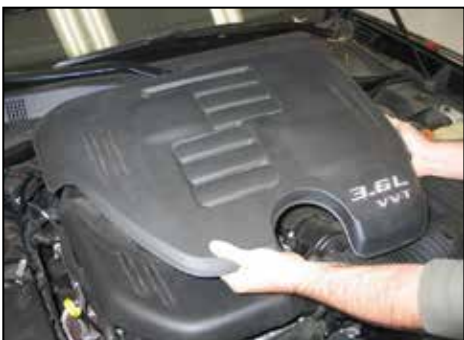
2. Lift up and remove the engine cover and remove it from the engine.
