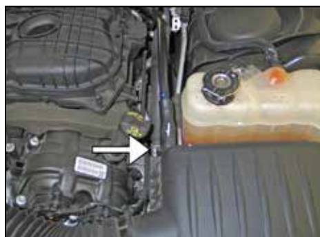
4. Disconnect the crankcase vent hose from the air filter housing.
