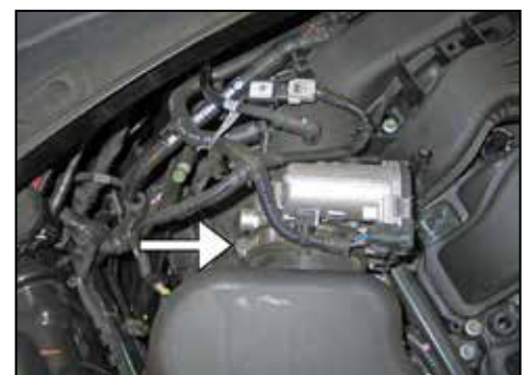
5. Loosen the hose clamp that secures the intake tube to the throttle body.
