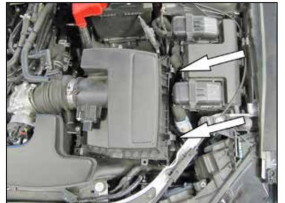
5. Release the two upper housing clips and then remove the upper housing, intake hose and air filter from the vehicle.
