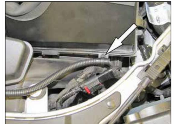
21. Connect the extension harness into the factory harness and then secure the harness to the lower air housing with the mounting tie wrap as shown.
