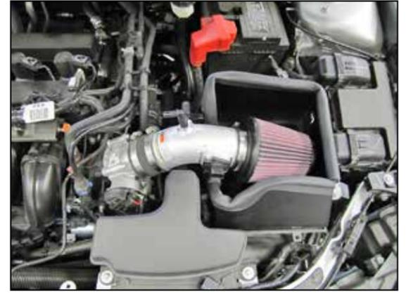
17. Install the Intake tube assembly into the silicone hose at the throttle body as shown, align for best fit and then secure with the provided hose clamp.
