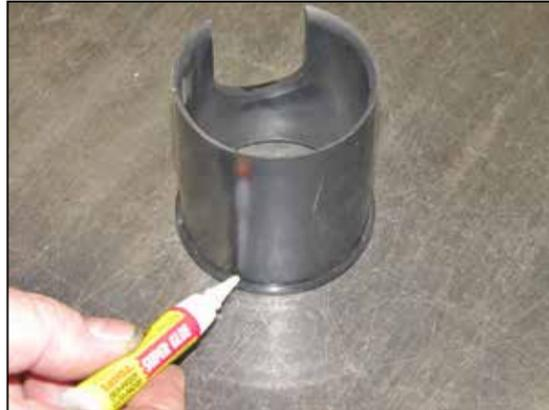
14. Apply several drops of the provided glue to the lip of the venturi insert as shown.
