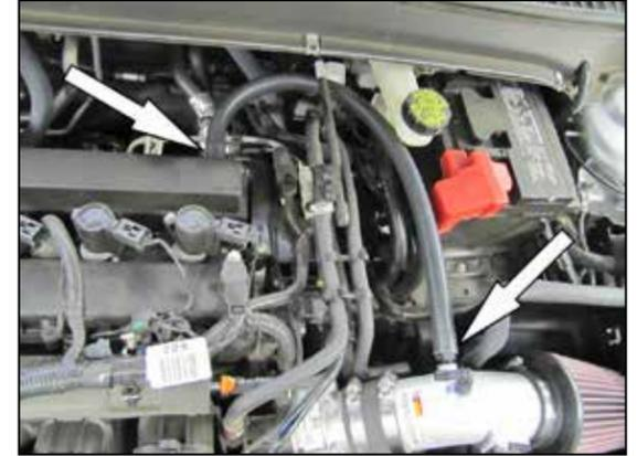
18. Install the provided crankcase vent hose onto the valve cover port and then onto the fitting installed into the K&N® intake tube as shown. **NOTE: Some trimming of the hose may be necessary.**
