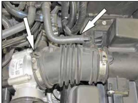
3. Disconnect the EVAP vent hose from the factory 90° fitting and then loosen the hose clamp securing the factory intake hose to the throttle body.
