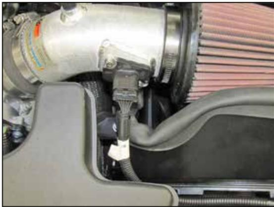
22. Connect the open end of the harness to the mass air sensor as shown.
