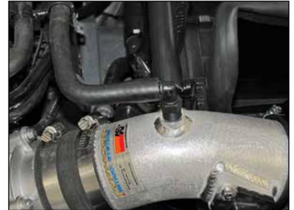
19. Connect the EVAP vent line to the 90° fitting installed into the K&N® intake tube as shown.
