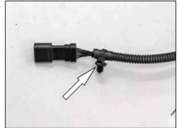
20. Install the provided "Mounting Tie Wrap" onto the female end of the mass air extension harness as shown.
