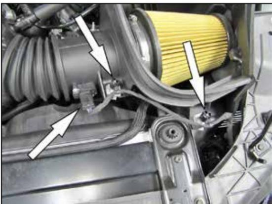
2. Disconnect the mass air sensor electrical connection and unhook the wiring harness from the mounting studs.
