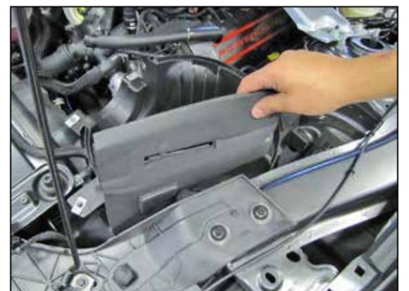
6. Remove the foam air dam from the inner fender.
