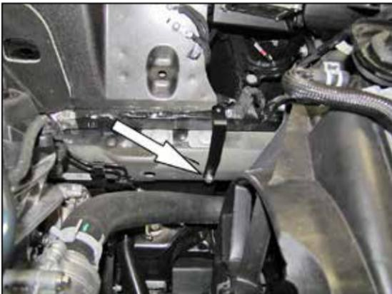
10. Install the heat shield mounting bracket (064325)
