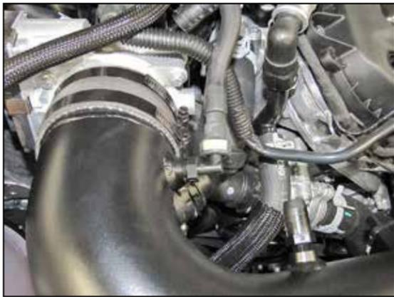
22. Connect the EVAP vent line to the quick disconnect fitting installed into the K&N® intake tube.
