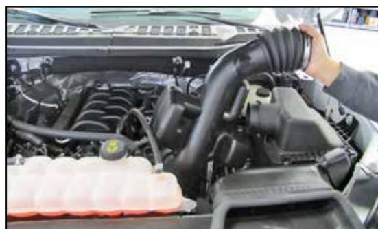
4. Unhook the coolant line from the intake tube and then remove the intake tube from the vehicle.
