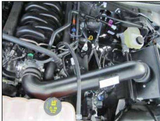
14. Install the K&N® intake into the coupling hose at the filter adapter and then into the hose at the throttle body, adjust the tube for best fit and then secure with the provided hose clamps.
