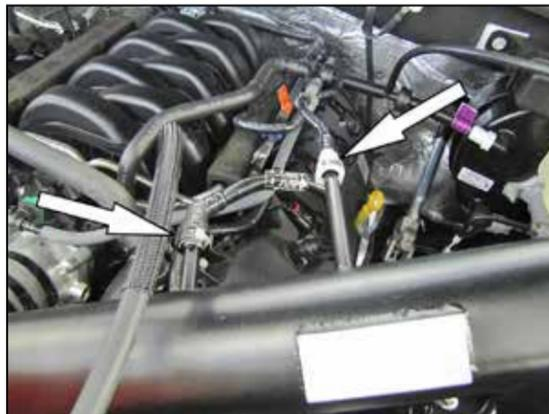
15. Connect the factory EVAP and Crank case vent lines to the fittings on the K&N® intake tube.
