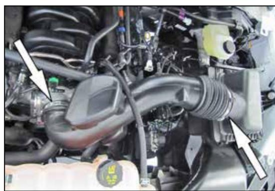
3. Loosen the hose clamps at the throttle body and filter inlet that secure the factory intake tube.
