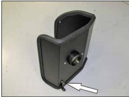
12. Install the provided heat shield mounting bracket (070015) onto the heat shield as shown using the provided hardware.
