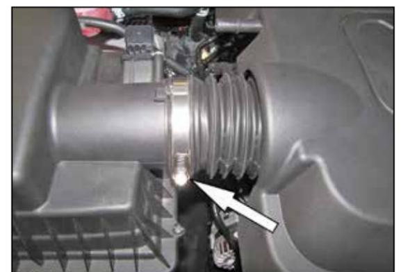
4. Loosen the hose clamp that secures the intake tube to the air filter housing.
