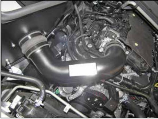
21. Install the K&N® intake tube into the hump coupler and then into the step coupler at the throttle body, adjust the tube for best fit and then secure with the provided hose clamps.
