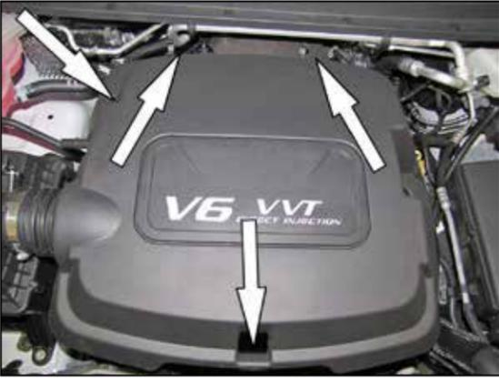
6. Loosen the two bolts that secure the rear off the intake plenum and remove the two forward bolts that secure the plenum.
