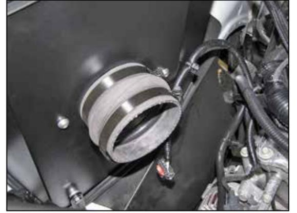
16. Install the provided hump coupler (06899) onto the filter adapter and secure with the provided hose clamp.
