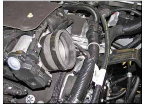
17. Install the provided step coupler (08186) onto the throttle body and secure with the provided hose clamp.
