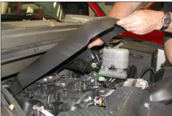
2. Remove the 8mm bolt that retains then engine cover onto the engine then remove the cover from vehicle.
