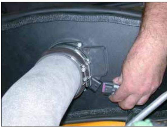
23. Reconnect the mass air electrical connection as shown.
