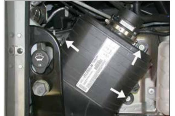
7. Remove the 3 10mm bolts that retain the air box onto the vehicle.
