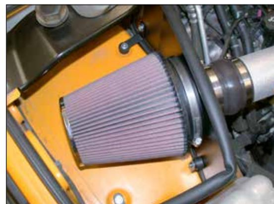
22. Install the air filter onto the mass air sensor and then tighten hose clamp.
