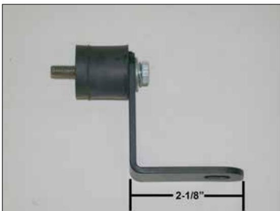
13. Install the 1" long rubber mounted stud (070226) onto bracket as shown.
