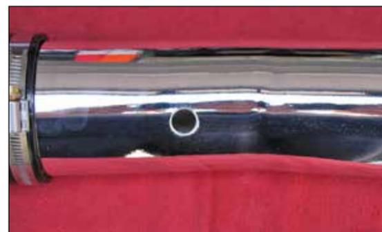
20b. Drill a 5/8" id hole at the location marked on the intake tube during the previous step. Be sure to remove any burrs or shavings after drilling the hole into the intake tube.
