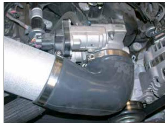
21. Tighten the hose clamp, which secures the silicone hose to the throttle body.
