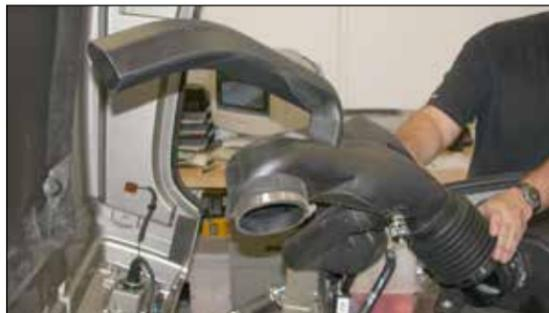
6. Detach the intake tube from the throttle body and mass air sensor then remove the intake assembly.
