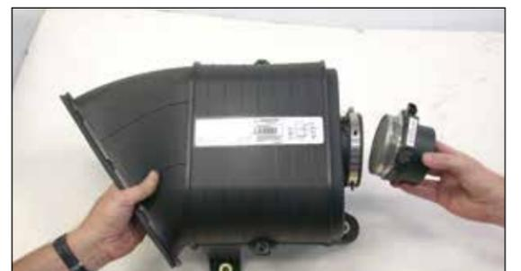
9. Loosen the hose clamp that retains the mass air sensor onto the air box then remove the mass air sensor from the air box.
