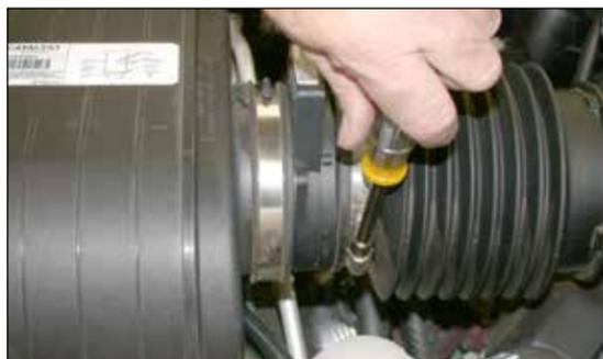
5. Loosen the hose clamp at the mass air sensor.
