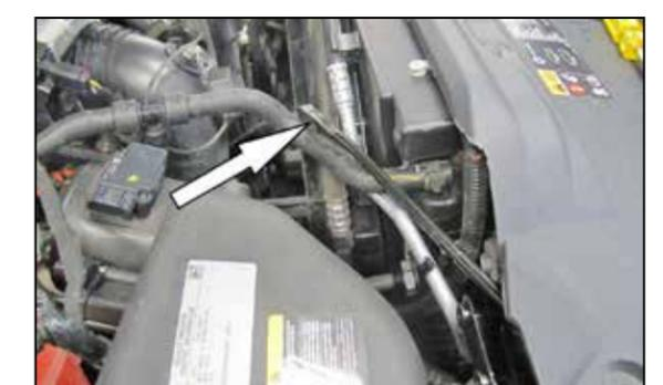
5. Loosen the bolt securing the fender brace to the core support then swing the brace clockwise towards the radiator for clearance.
