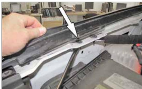
4. Lift up the hood seal trim and remove the bolt securing the fender brace.
