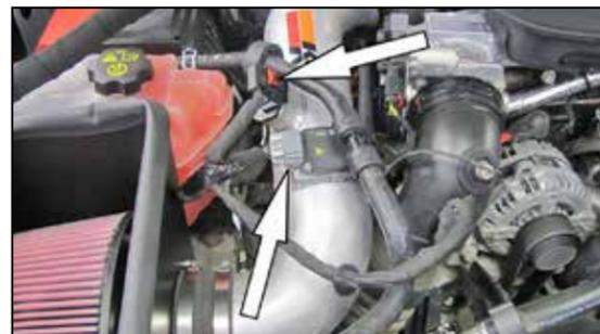
18. Reconnect the Mass air sensor and humidity sensor electrical connections.
