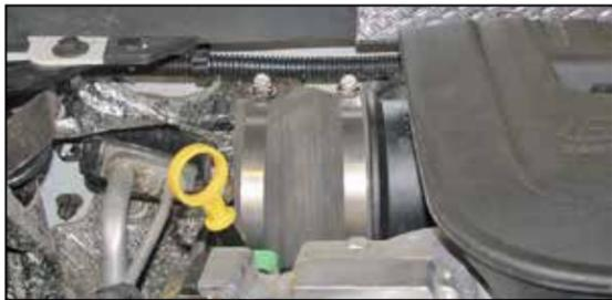
13. Install the provided coupling hose (08633) onto the turbo inlet and secure with the provided hose clamp.
