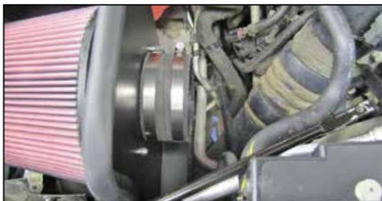
12. Install the coupling hose (08761) onto the filter adapter and secure with the provided hose clamp.
