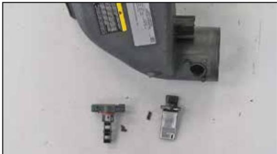
14. Remove the screws securing the mass air sensor and Humidity sensors into the factory air box and then remove the sensors from the air box.
