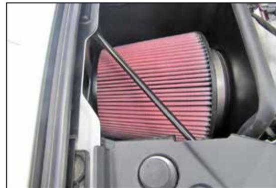
19. Reinstall the fender brace and secure with the factory hardware.
