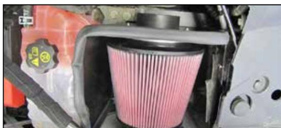
11. Flex the heat shield back and then install the K&N® air filter onto the filter adapter and secure with the provided hose clamp. Secure the heat shield with two of the factory bolts removed in step #7.
