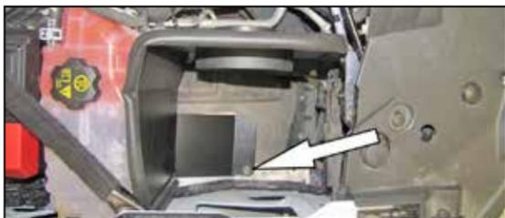
10. Install the heat shield assembly into the vehicle and secure with one of the factory bolts removed in step #7 to the fender.
