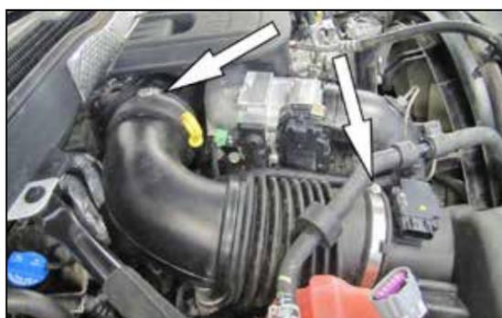
3. Loosen the hose clamps securing the factory intake hose to the air box and turbo inlet.
