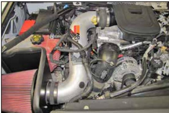
17. Install the K&N® intake tube into the hump hose at the turbo inlet and then into the hose at the filter adapter, adjust the tube for best fit and then secure with the provided hose clamp.
