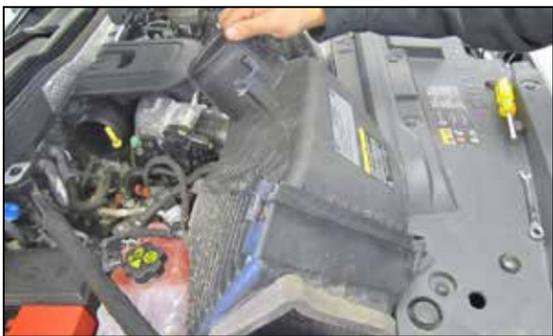
6. Lift up and remove the air box from the vehicle.
