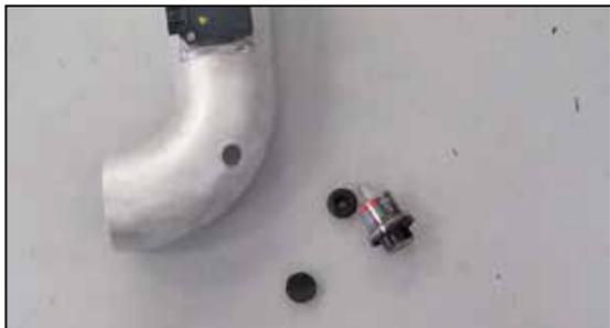
16. On vehicles equipped with a filter minder, remove the filter minder and grommet from the factory air box and install them into the K&N® intake tube. On vehicles not equipped with a filter minder, install the provided plug into the K&N® intake tube.
