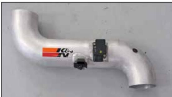
15. Install the mass air sensor and humidity sensor into the K&N® intake tube and secure with the provided hardware.
