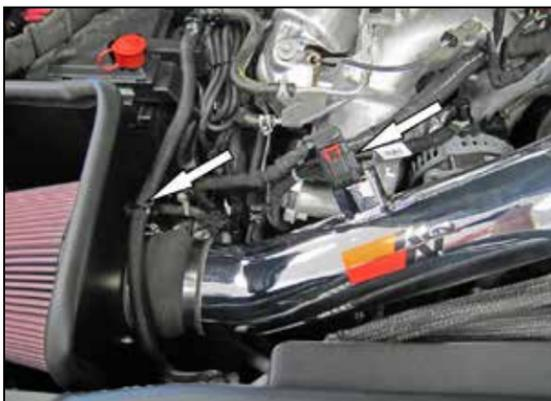
14. Reconnect the mass air sensor electrical connection and secure the coolant bypass hose to the heat shield using the factory retaining clip.
