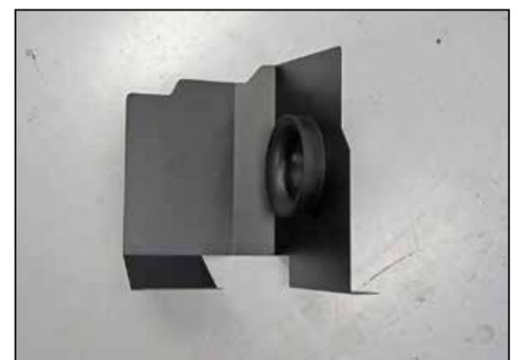
6. Install the provided filter adapter into the K&N® heat shield and secure with the provided hardware.
