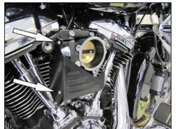
6. Install the K&N® servo cover and secure with the provided hardware to the original servo cover mounting bolt locations.
