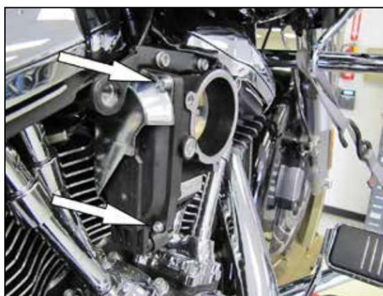
5. Remove the two servo cover bolts shown.
