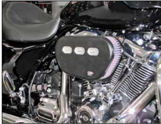
12. Install the filter and top plate and secure with the provided hardware from the back side.
